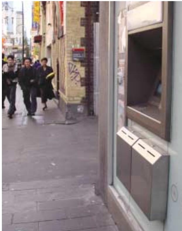
Protrusion of the sharp rubbish containers inhibits and endangers the vision impaired.
