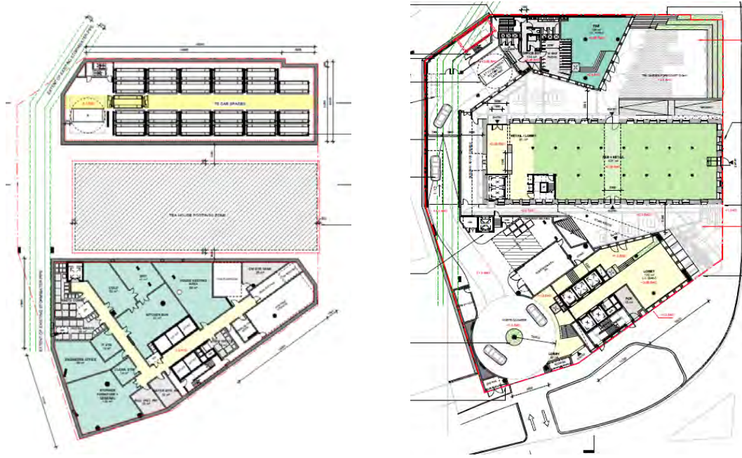
Figures 24 and 25: Basement showing provision for 70 spaces in stacker system to the north (left) and ground floor vehicle access (right) (Source: Applicant)
