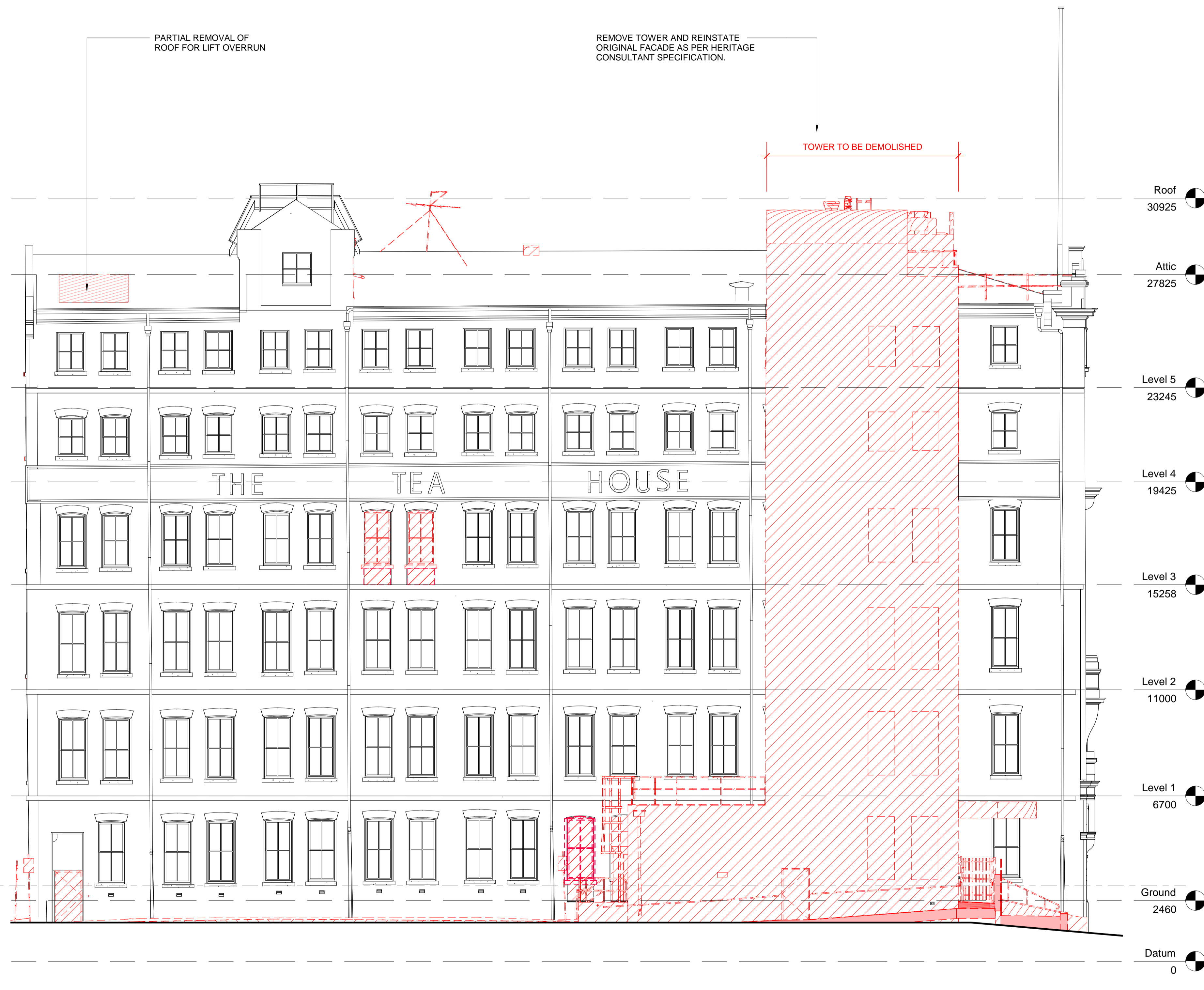
2 SOUTH DEMOLITION ELEVATION 1 : 100
