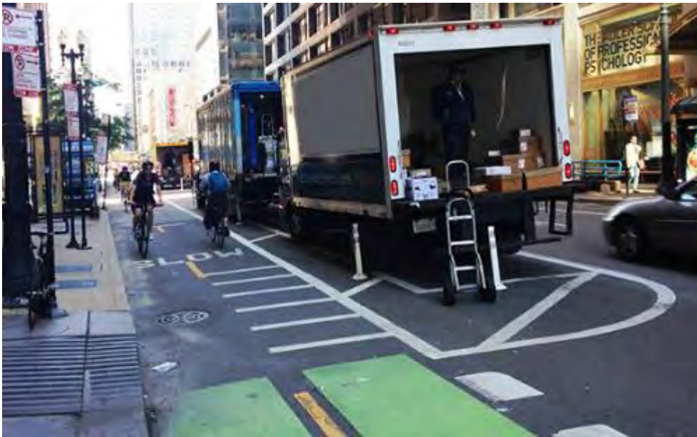
Floating loading zone for several trucks, Chicago
