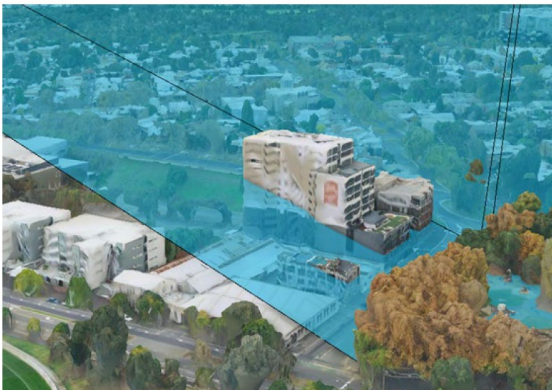
Figure 2 Figure showing how the maximum developable volume of a property can extend into a park's solar volume
