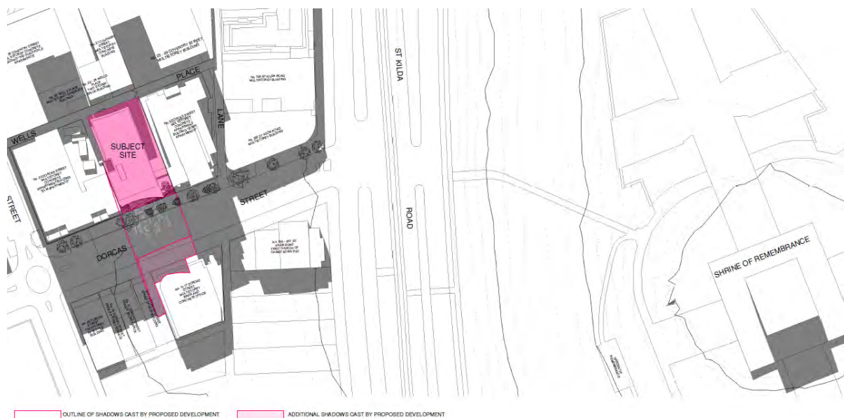
Figure 10: Diagram showing extent of shadows cast by development at 2pm on 22 September. 22 April shadows comparable. (source: application plans prepared by Plus Architecture)
