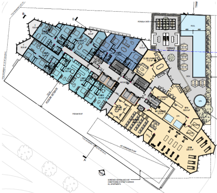
Figure 4 - Level 06 (podium rooftop) showing residential amenities and the triangular form of the tower above (source: application plans prepared by Rothe Lowman)
