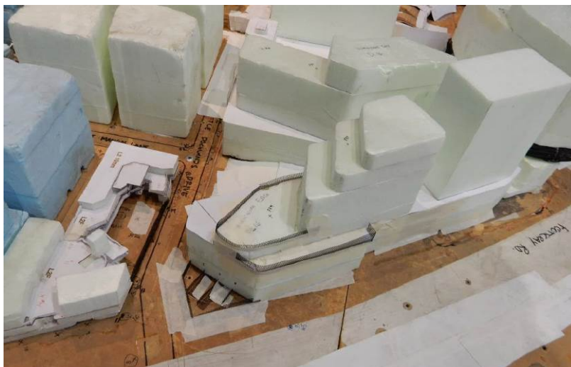
Figure 32 – Wind tunnel model showing mitigation screens and exclusion zone (MEL Consultants Report, dated 21 June 2020)
