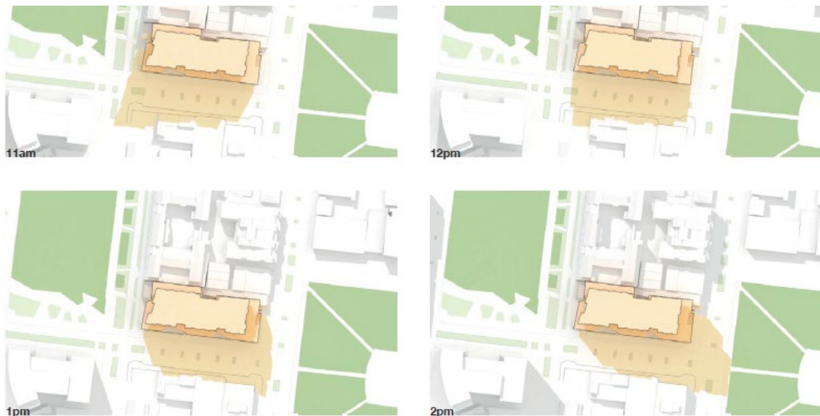
22 September shadow diagrams (11am to 2pm) note the overshadowing to the footpaths on the north and south sides of Pelham Street
