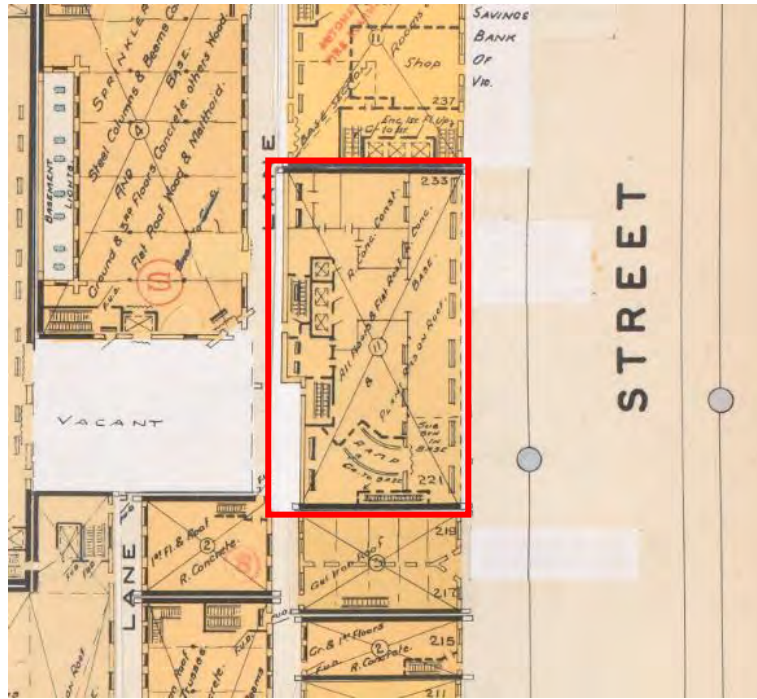
Figure 2. Detail from Mahlstedt fire survey plan dated 1948, and presumably amended in the 1970s, shows the subject building as an 11-storey building with basement of reinforced concrete construction. (Mahlstedt Map Section 1, no 16, 1948).
