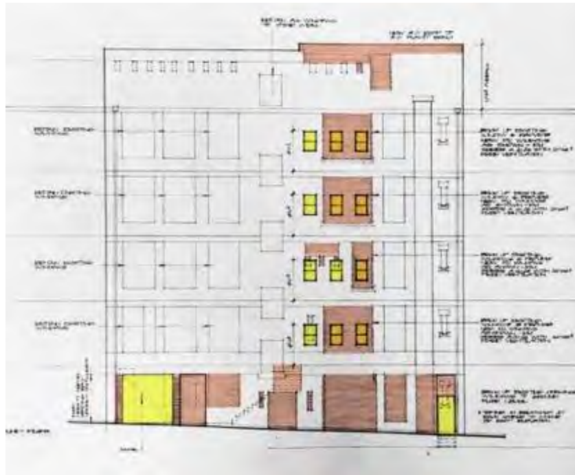
Figure 5. East (Melbourne Place) elevation drawn by Meldrum Burrows & Partners in 1972. Coloured in orange are original openings to be bricked and coloured in yellow are new openings introduced to the rear elevation. (PROV Public Building Plan VPRS8044/P/3)
