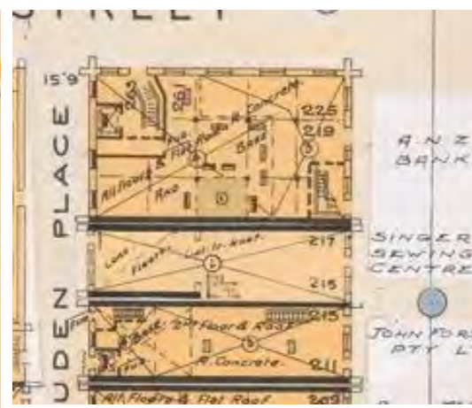
Figure 3. The 1948 Mahlstedt fire survey plan (amended in a later date), showing the shops at 215-217 Swanston Street extended to the western allotment boundary (Source: Mahlstedt Map section 1, no 10, 1948)
