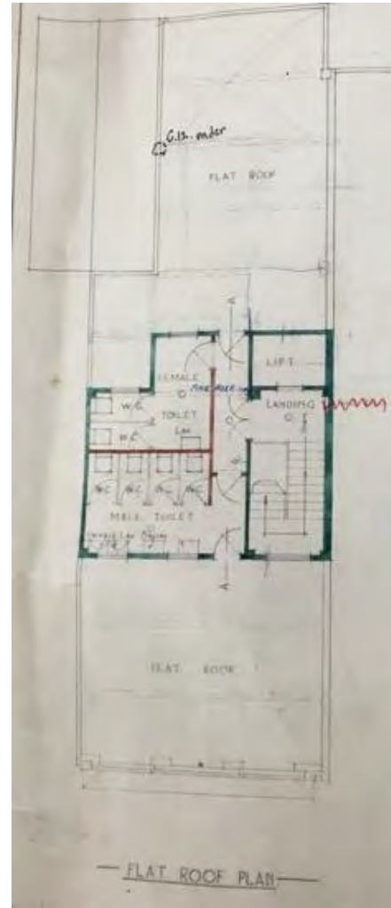
Figure 2. Original building plan with the 1927 addition of a concrete room on the roof drawn over top. (Source: PROV VPRS 11201/P1 unit 99, item 7871)
