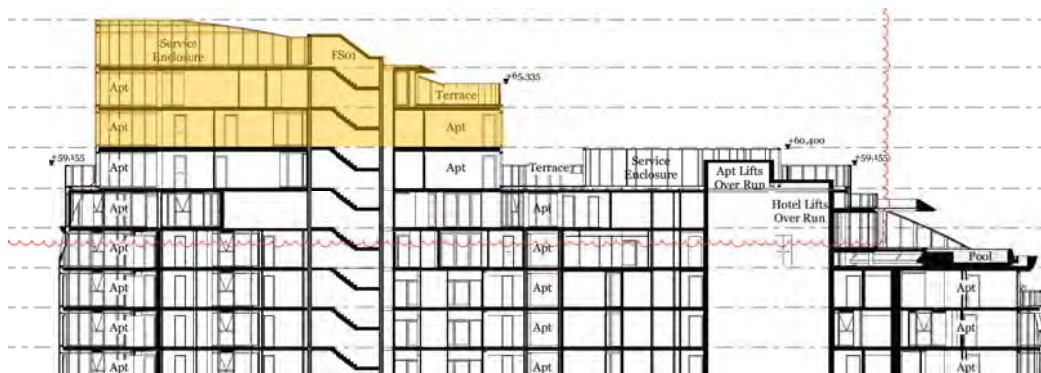
Figure 9 - Extract from Section AA, marked up to show additional height (shaded yellow). From Drawing TP304
