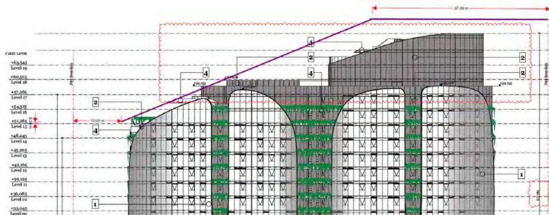
Figure 11 - East Elevation extract (Drawing TP300), marked up with the DP Addendum envelope (purple line)
