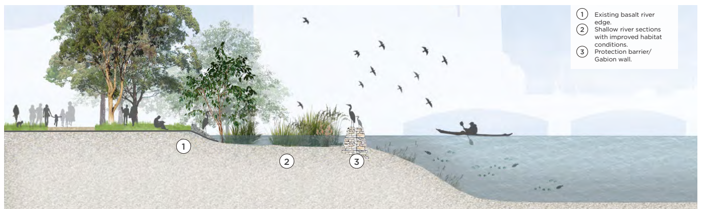
Image 65. Proposed river edge with extended riparian zone and replanting with indigenous species (Illustrative for discussion purposes only)
