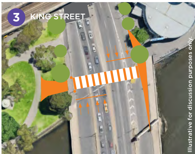
Image 96. Kings Street improved path and crossing alignment, kerb outstands and additional street trees (Illustrative for discussion purposes only).
