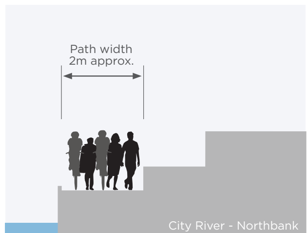
Image 93. Typical cross-section of Flinders walk, lower river path, highlighting the spatial constraints
