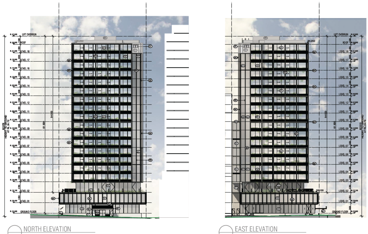
Figure 3: Proposed elevation plans depicting the proposed tower above the existing heritage building.
