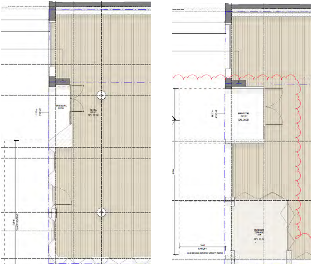
Figure 9 - Original (left) and revised (right) Ground Level Plan extract showing the Lygon Street interface. From Drawing A1.01
