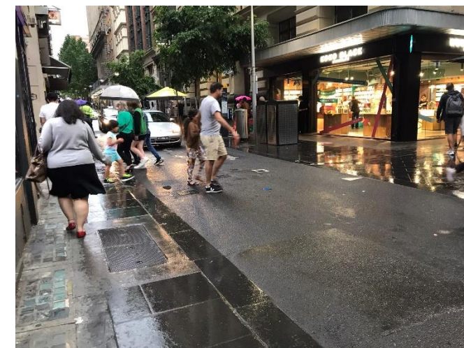
Raised section of Flinders Lane without colour or texture contrast, Melbourne CBD
