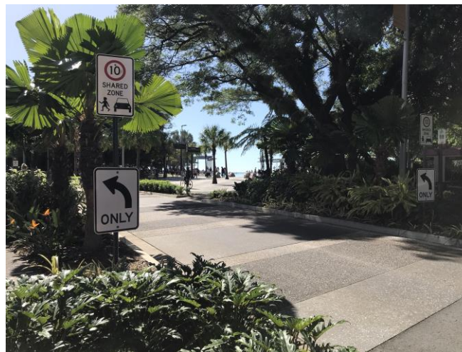
Threshold at entry to shared zone with surface colour and texture change and street narrowing, Cairns, QLD
