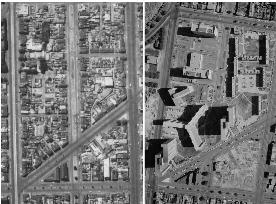
Figure 17 Aerial photograph of the Carlton HCV estates, 1951 (left) and 1969 (right), showing earlier buildings replaced with low-rise walk up blocks and high-rise tower blocks Source: Land Victoria Historic Aerial Photography Collection
