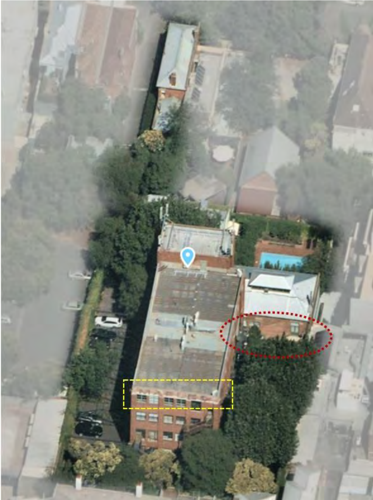
Figure 12. Birds eye view of the subject site, looking west. Note the remnant painted sign on the east elevation of the 1922 former storage building, highlighted in yellow dashed line. The window openings on the former grain store shown in dashed lines are not original, highlighted in red dashed line. (Source: Nearmap 2022 with GML overlay)
