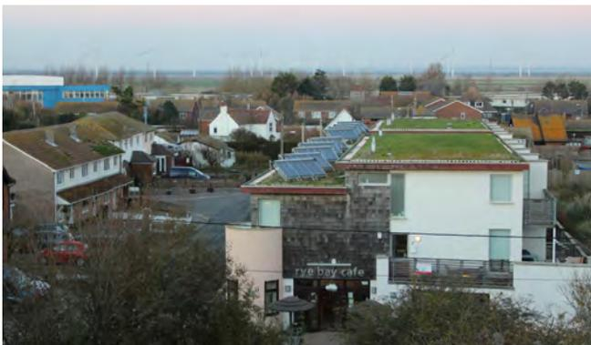
Figure 22. Biodiverse extensive green roof at Lydd Road, Camber, UK.
