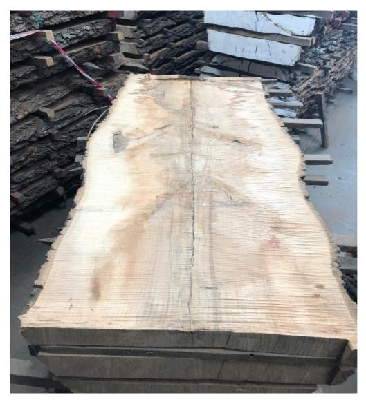
Timber Lot ID #1 - Narrow-leaved Ash milled timber slabs.
