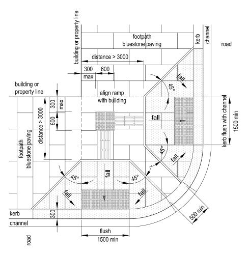
300 x 300mm 'Versatac' granite hazard TGSI's installed on 25mm bedding mortar. Hazard TGSI's shall be installed perpendicular to the pedestrian line of travel.
