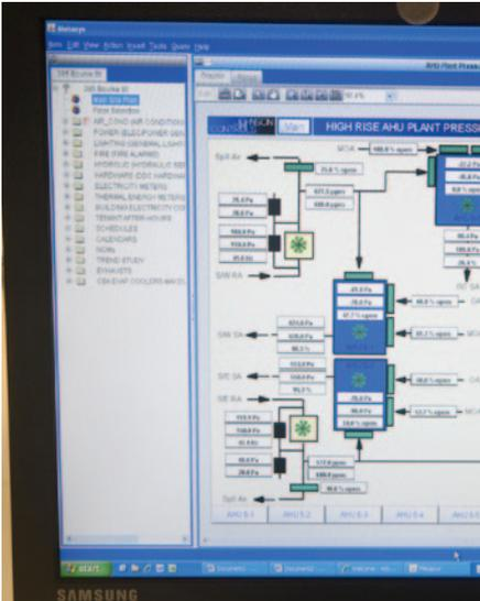
Key sensors to the control systems (supply air temperature and system pressure) were recalibrated and relocated to improve reliability and accuracy.
