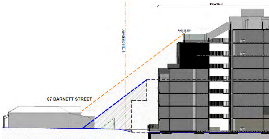
Figure 36 - Shadow Diagram extract, showing that the rear yard of 87 Barnett Street is already completely overshadowed at 9am on the Equinox. From Drawing TP08.05
