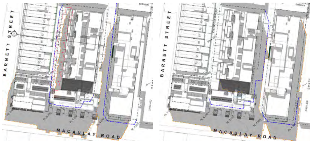
Figure 34 - Shadow analysis showing proposed shadows at 11am (left) and 2pm (right). From Drawings TP08.06 & TP08.07
