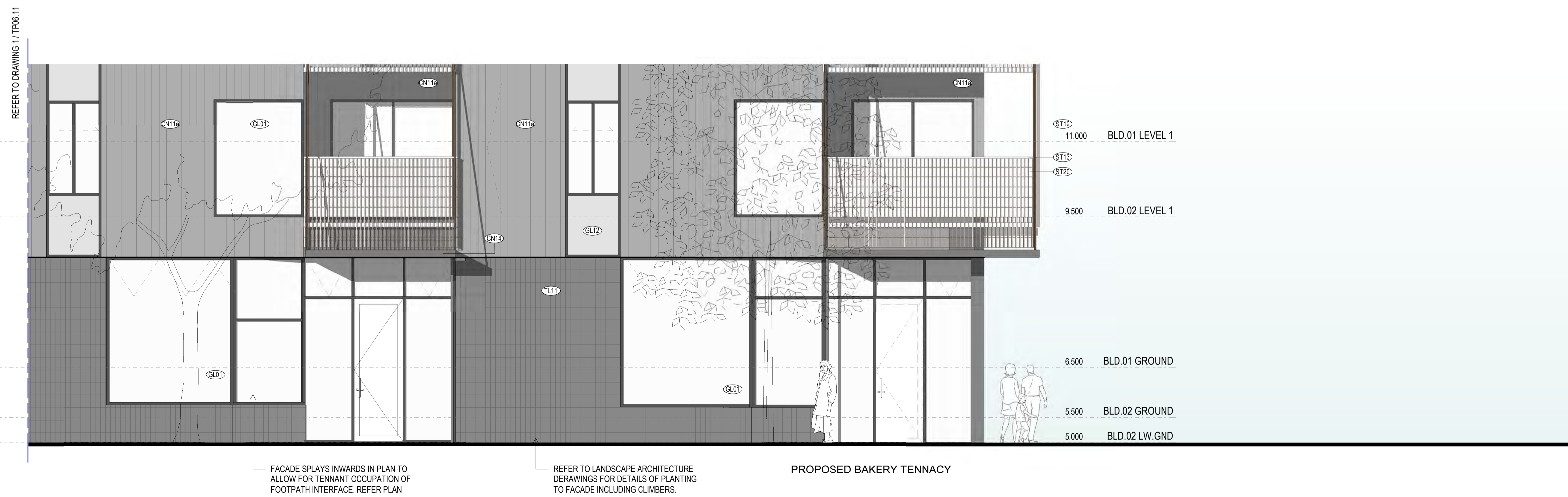
2 RETAIL FRONTAGE ELEVATION - BUILDING 02 SOUTH 02 1:50
