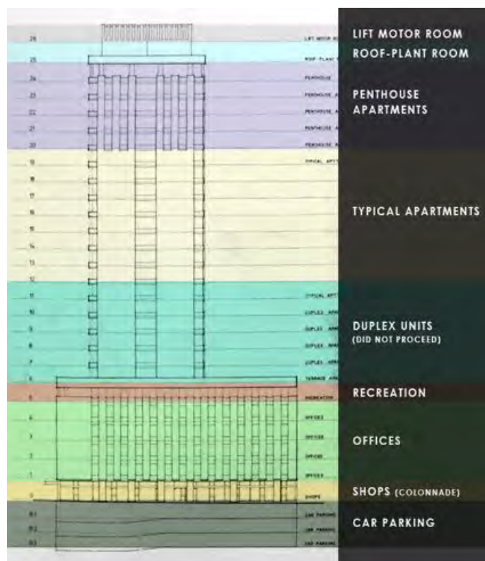
Figure 1. The development plan for 93-101 Spring Street, with floor levels coloured over the elevation plan in different shades as per proposed uses (Source: J V Edgar Pty Ltd c1969:9).
