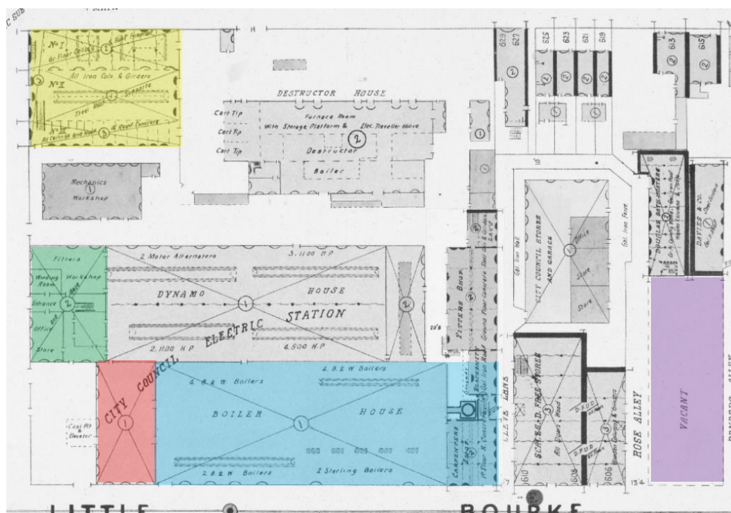
Figure 5. By the latter half of the 1920s, Substation J (shaded yellow) was built on the corner of Spencer and Lonsdale streets. The brick workshops were built on the eastern portion of the site at 620-648 Little Bourke Street (shaded blue). The Offices building (shaded green), the Economiser building (shaded red), and the vacant yard at 602-606 Little Bourke Street (shaded purple) remained unchanged since 1910. (Source: Mahlsted Map Section 1, no 22, 1925 with later additions)
