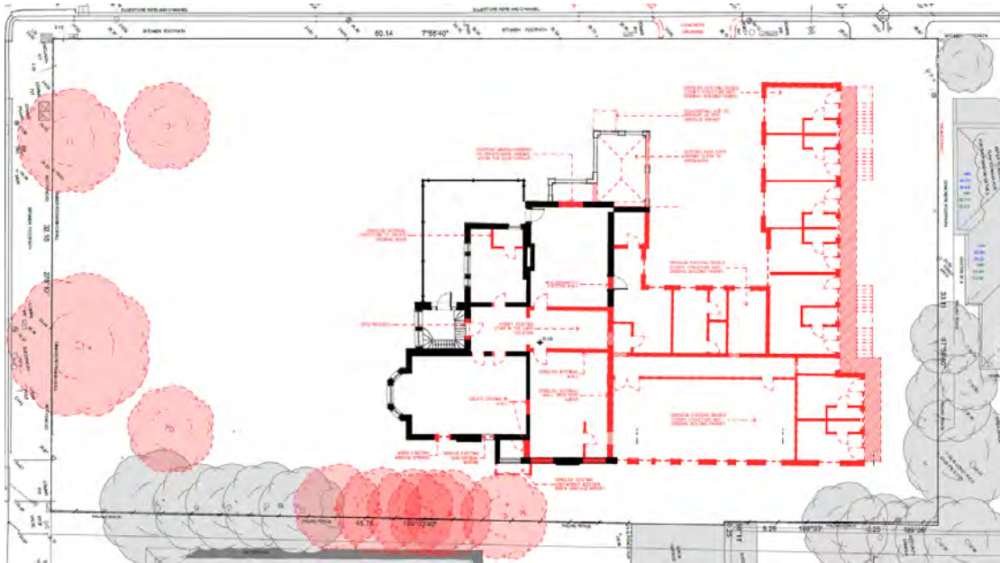
Figure 7: First floor demolition plan (Source: Applicant)
