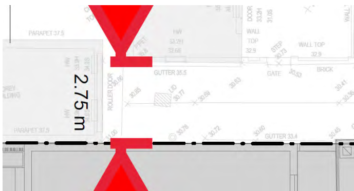
Figure 30 – extract of the site plan showing the subject habitable room window and the setback to the proposal across Von Guerard Place (Source: applicant, dimension by Council)
