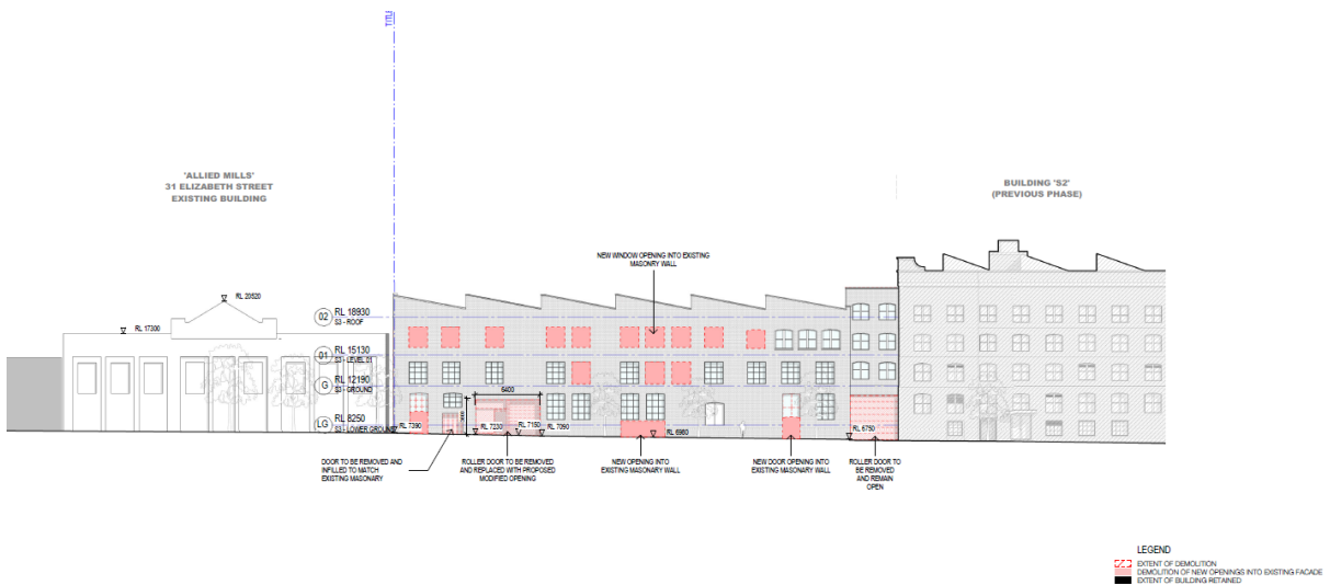
Excerpt from 'Demolition – Elevation East – Elizabeth Street', Drawing No. SK 2 3200, Rev B
