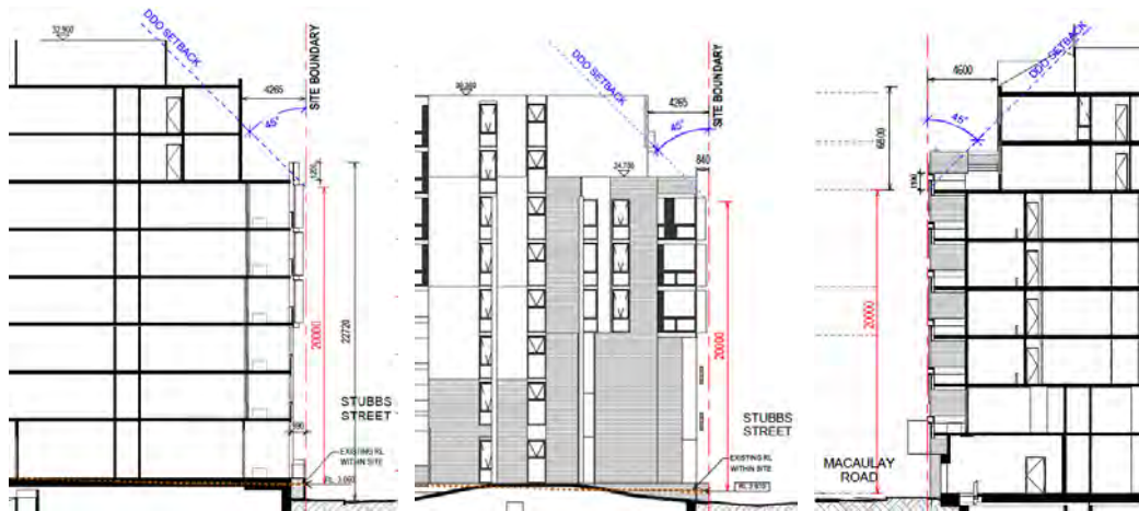
Figure 13 - DDO63 Setback line depicted on Buildings A, C & D. From Drawing TP07.01.
