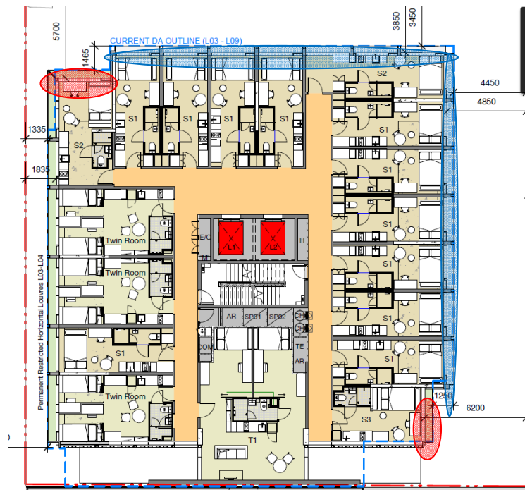
Figure 7: Typical proposed floor layout plan. Blue circle denotes the primary element and the red circle denotes the secondary element.
