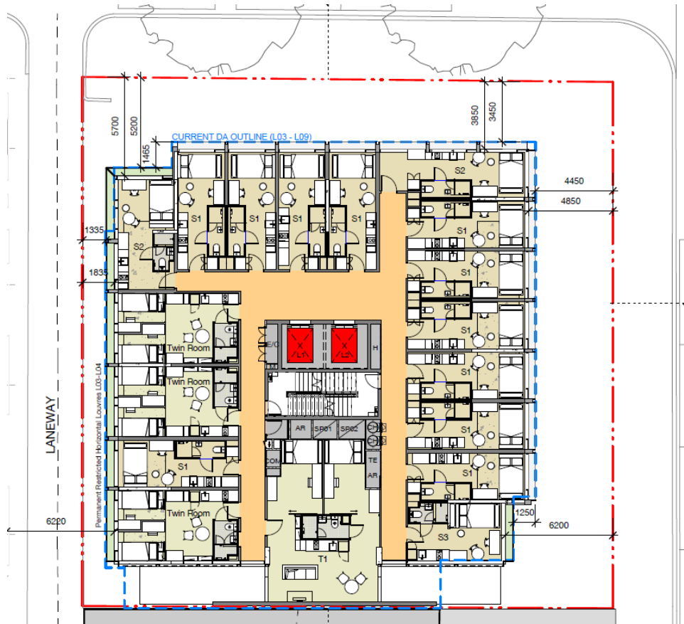
Figure 6: Typical proposed floor plan. The blue line denotes the approved development outline.
