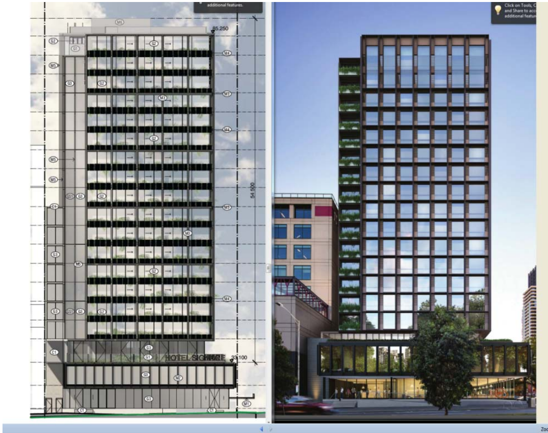
Figure 4: The image to the left is the approved east elevation. The image to the right is the proposed east elevation plan.
