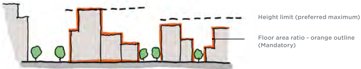
Figure 2.2: Floor area ratios help to control the density, or intensity, of the development in relation to the size of a site. The orange outline above highlights a potential allowed density of a site according to an floor area ratio control. When used in combination with design objectives such as setbacks, floor area ratios can enable a better response to the surrounding context and character of a site, allowing for a greater diversity of buildings while placing a natural cap on height.
