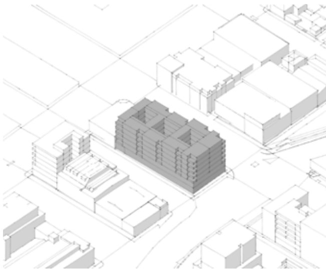
Figure 3.33: Built form testing to show the proposed floor area ratio and built form controls on a large corner site in Station Precinct (DDO28). Images are indicative only to test the proposed controls and are not representative of actual building proposals ( West Melbourne Built Form Testing , Breathe Architecture).
