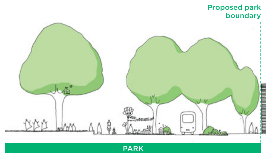
Section A: Proposed conditions of Leicester Street looking north towards Grattan Street showing the park extending to the building edge, wide pedestrian paths and a single northbound traffic lane 'road within a park'
