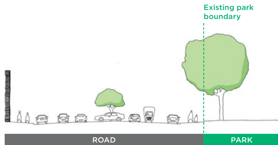
Section A: Existing conditions of Barry Street looking north towards Grattan Street showing the car-dominated street and poor relationship to the park
