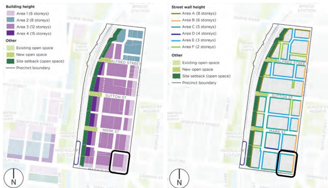
Figure 122 - Preferred Maximum Building Height (left) and Street Wall Height (right) maps from the proposed DDO75
