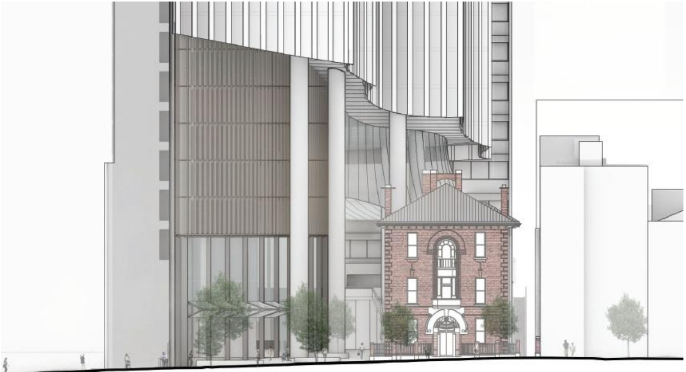
Excerpt from Urban Context Report (Issue A) showing 'Revision G' façade design of proposed Tower 2, with removal of overhang over Milton House (p.64 of 94)
