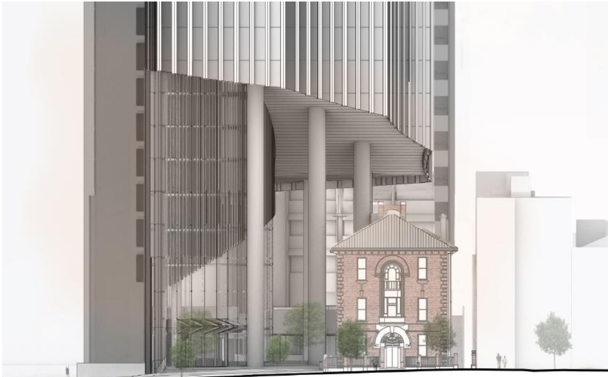
Excerpt from Urban Context Report (Issue C) showing ‘Revision J’ façade design of proposed Tower 2, with reintroduction of overhang over Milton House (p.78 of 107)
