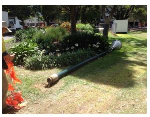
Cause: Truck reversed into light pole
