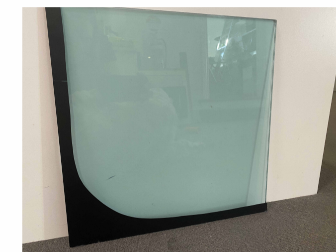
1:1 SAMPLE OF MATT BLACK VINYL DECAL TO CORNERS OF WINDOWS AT ENTRY TO CREATE SOFT ROUNDED EDGES
