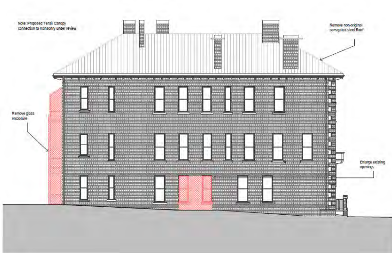
East Elevation (Demolition) Sc. 1,100
