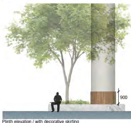
Plinth elevation / with decorative skirting
