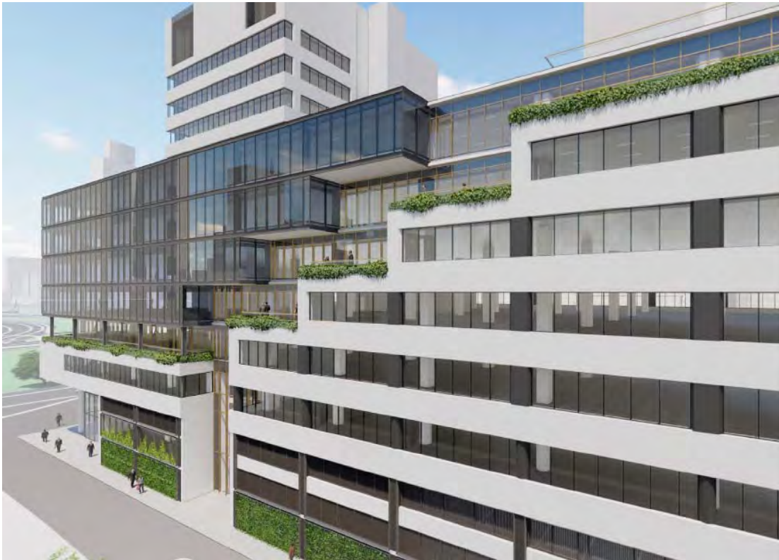
Figure 12 - 3D Render showing proposed extension (curtain wall glazing) in relation to the existing street wall (white concrete and glazing)
