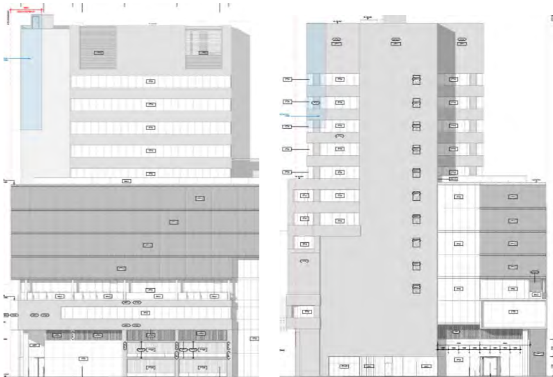
Figure 14 - Proposed North (left) and East (right) Elevations depicting extent of non-compliance of existing building with the setback requirements of DDO10
