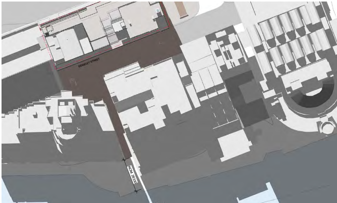
Figure 18 - Winter Solstice Shadow Diagram, confirming that the shadow at 2pm would fall approximately 28 metres short of the north bank of the Yarra River
