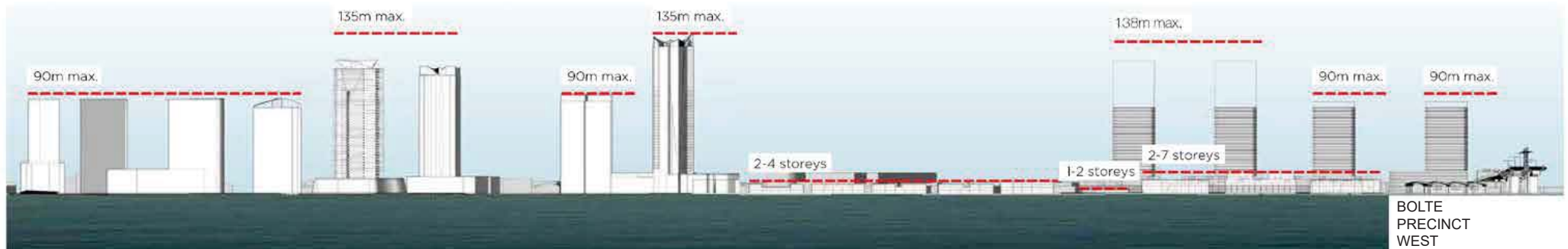
Comparative Building Height Elevation. Diagram from Yarra's Edge Western Precinct Development Plan, 2013.
