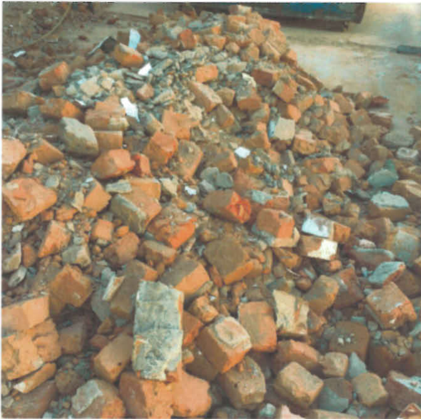
View of removed bricks – many cracked, broken and half bricks.
