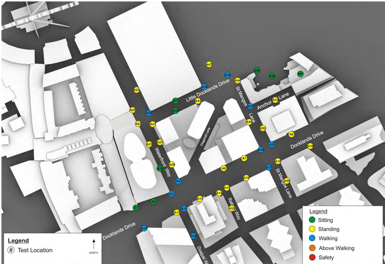
Figure 6a – Summary of wind conditions for the Existing Configuration for 360° of wind direction
