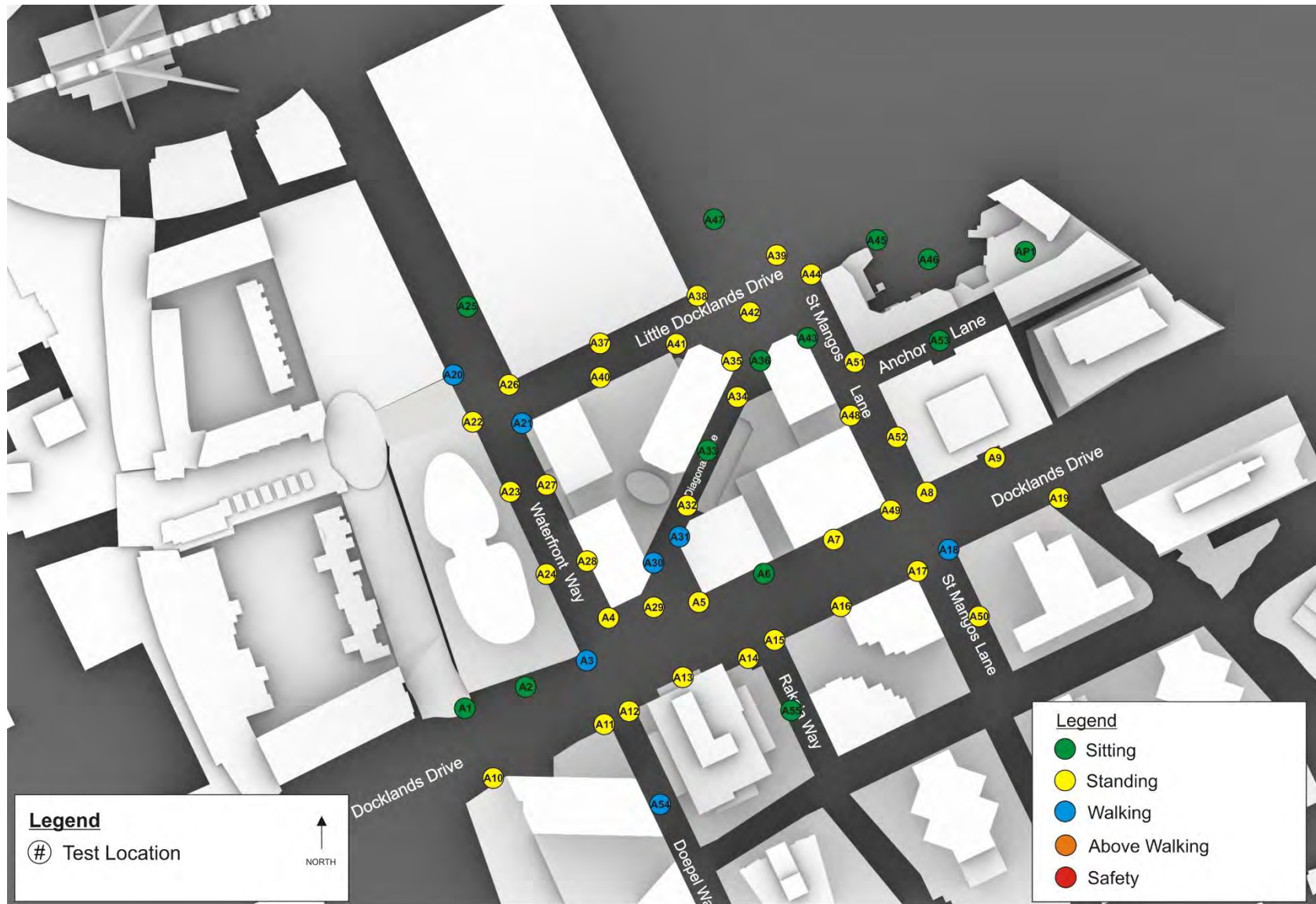
Figure 6b – Summary of ground level wind conditions for the Proposed Configuration for 360° of wind direction
