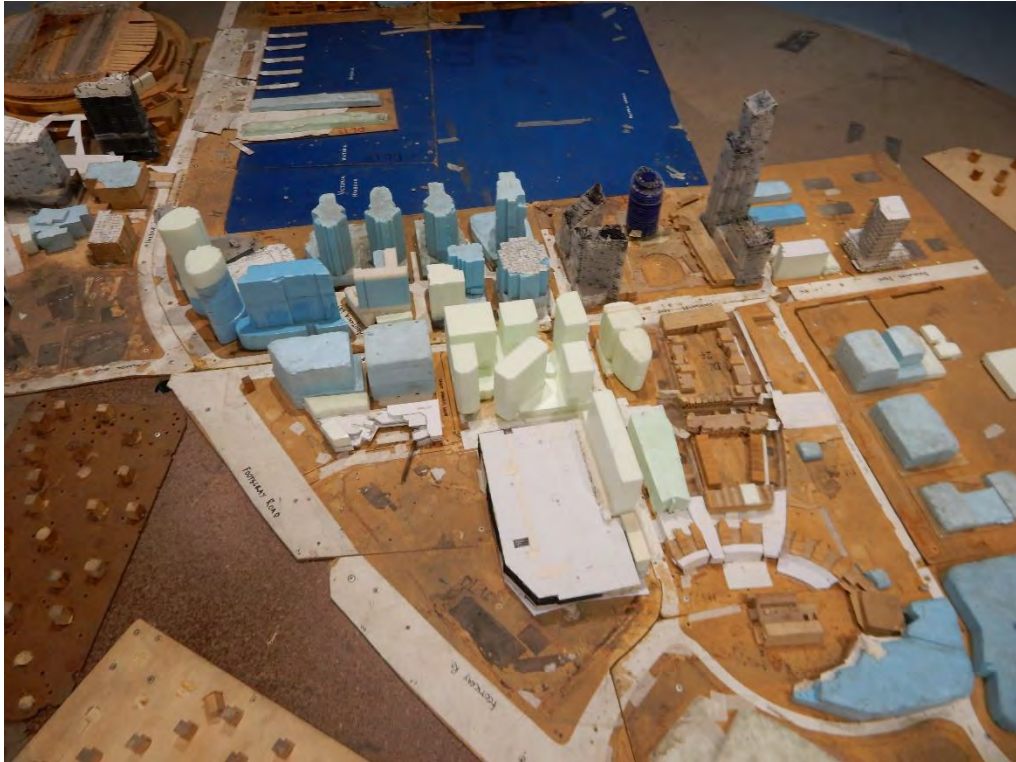
Figure 3 – View from the north of the 1/400 scale model of the 396-400 Docklands Drive, Docklands in the wind tunnel.
