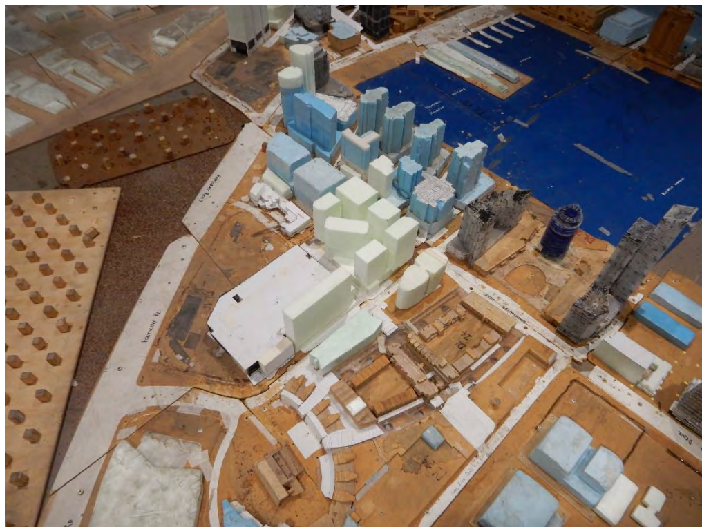
Figure 4 – View from the northwest of the 1/400 scale model of the 396-400 Docklands Drive, Docklands in the wind tunnel.
