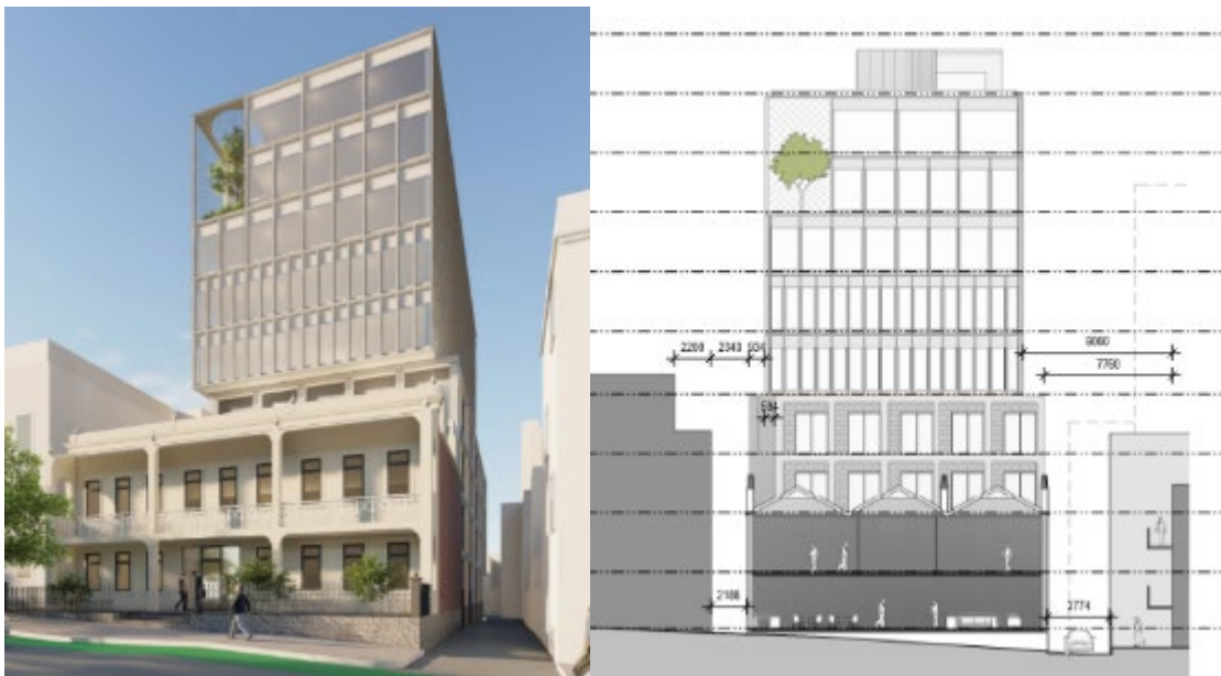
Above: Render of the building considered by VCAT (left) and cross section through the front section of the retained building (right) (Source: Amended VCAT plans)
