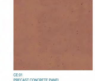
PRECAST CONCRETE PANEL Precast concrete panels with oxide pigmented finish. Colour to match MA:01
