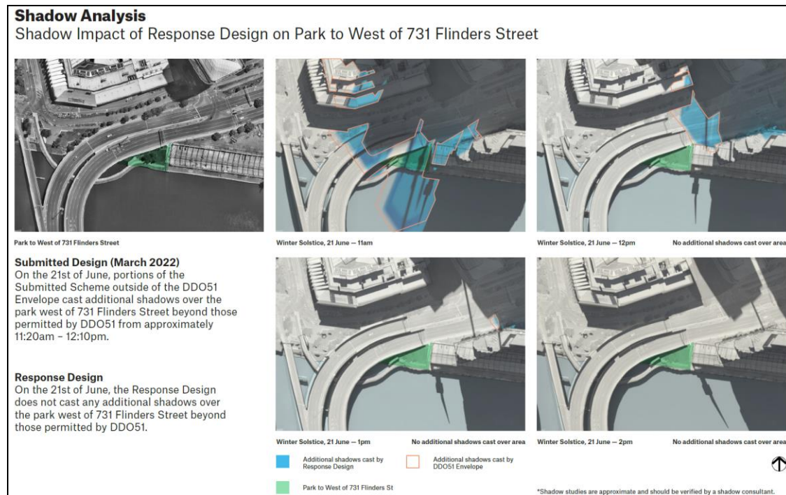
Figure 31: Shadow diagrams on 21 June showing shadows cast in relation to the park located to the west of Seafarer's Rest
