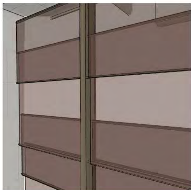
ST-01 Perspective of Albert Street Portico Screen. The design references both the datum lines of 366 Albert Street and the tripart composition of 364 Albert Street. MT-05 metal screen provides varying degrees of transparency in the rhythm of banding, providing views to the park while obscuring direct internal view.
