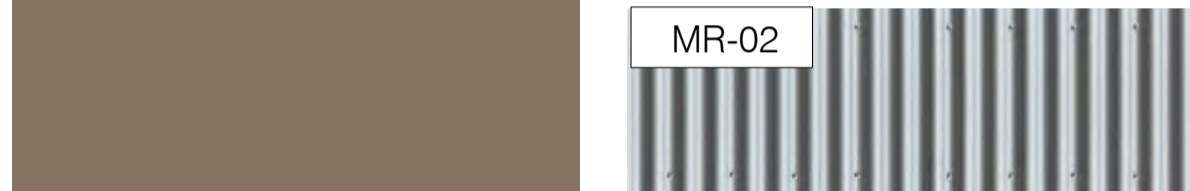
MR-02 New corrugated galvanised sheet metal to replace existing verandah T-PF-01 Paint finish to 364 Albert fretwork and faux metal work
