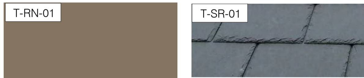
T-RN-01 Restored render finish to 364 Albert Street (Southern Elevation) T-SR-01 364 Albert Street roof to be re-clad in Welsh slate
