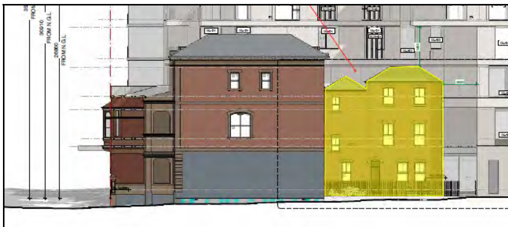
Figure 6: Rear service wing to be demolished and reconstructed (yellow)
