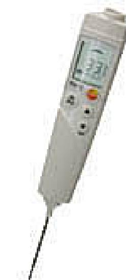
Provide a probe/stem thermometer capable of measuring temperatures to an accuracy of +/-1°C.
