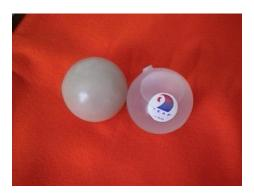
Figure 2 - PCM-filled Spheres (MJM Engineering)
