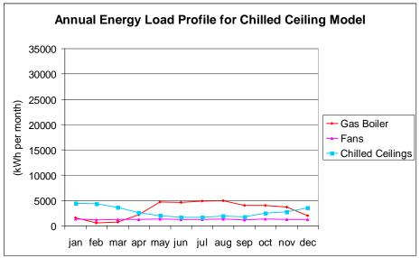
Figure 20. Estimated annual energy load profile for chilled ceiling model
