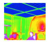
Figure 4. Chilled ceilings radiant cooling effects
