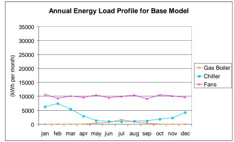
Figure 12. Annual energy load profile for the base model
