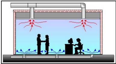
Figure 16. Displacement ventilation effects
