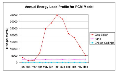
Figure 25. Estimated annual energy load profile for the PCM model
