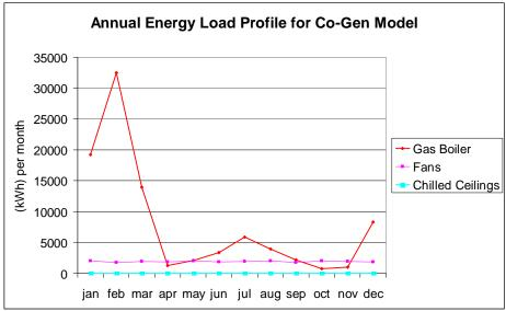
Figure 28. Estimated annual energy load profile for co-generation model
