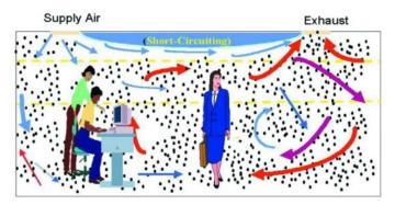
Figure 11. VAV system mixed air distribution
