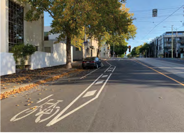
Figure 9: Example of non-physically separated kerbside bike lane - transition from mid-block treatment (top image) to intersection treatment (bottom Image)(Queensberry St, North Melbourne)
