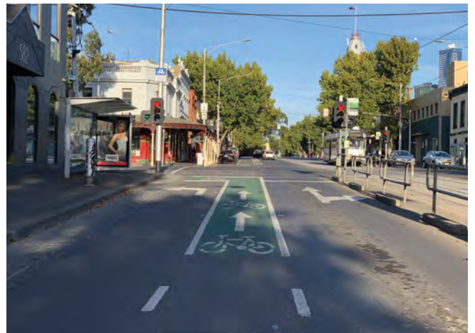
Figure 10: Example of Bike lane between left turn and through traffic lane - transition from mid-block treatment (top image) to intersection treatment (bottom Image)(Queensberry St, North Melbourne)
